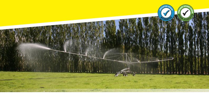
A very efficient, low cost, low pressure Travelling Irrigator.
